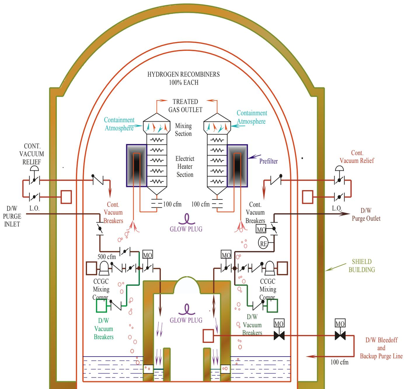
Figure 6.5-7 Mark III Containment Combustible Gas Control
