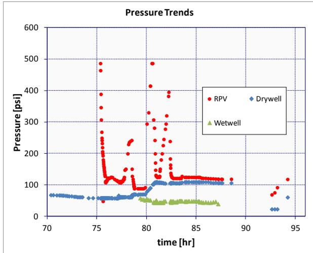
Fig. 1. Depiction of the available pressure data trends around the time of RPV depressurization to illustrate the large differential pressure between containment and the RPV at the time of depressurization.
