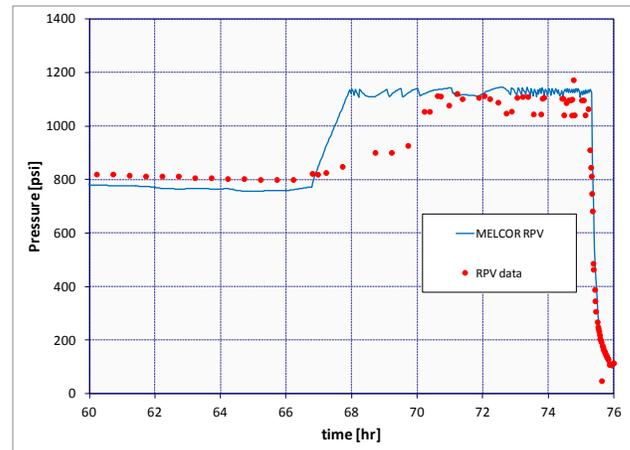
Fig. 6. Comparison of pressure data and the analysis predicted pressure for the RPV around the time of RCIC failure.
