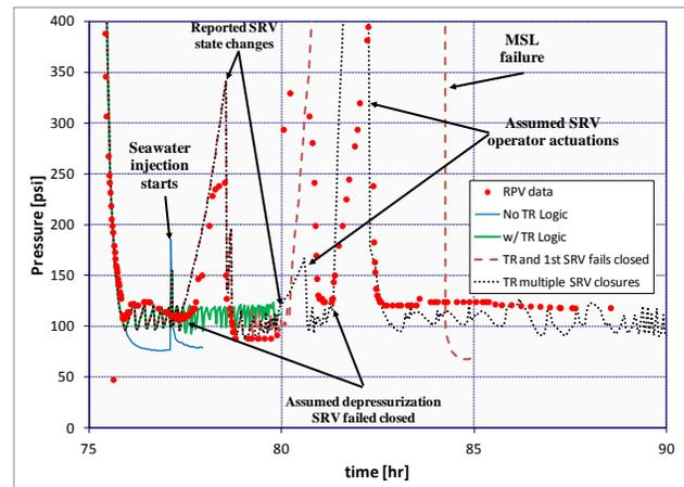
Fig. 7. Model development regarding the assumed SRV failures and operators actuations.
