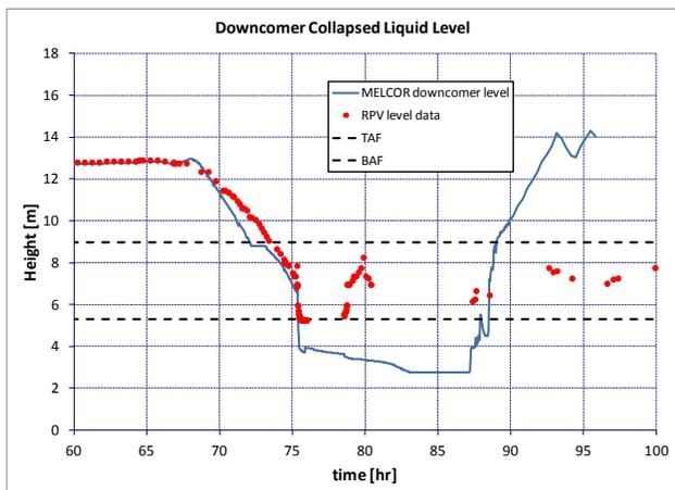
Fig 9. Comparison of the RPV level data and the analysis results for the collapse liquid level in the downcomer.
