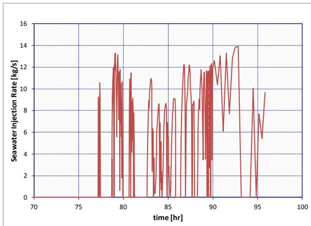
Fig. 8. Analysis predicted seawater injection rates when applying the assumed fire engine pump curve.
