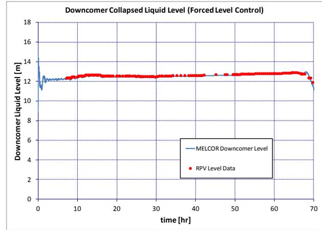
Fig. 5. Level indications are compared to the imposed RCIC controlled level. A zero level is equivalent to the base of the lower head of the RPV.
