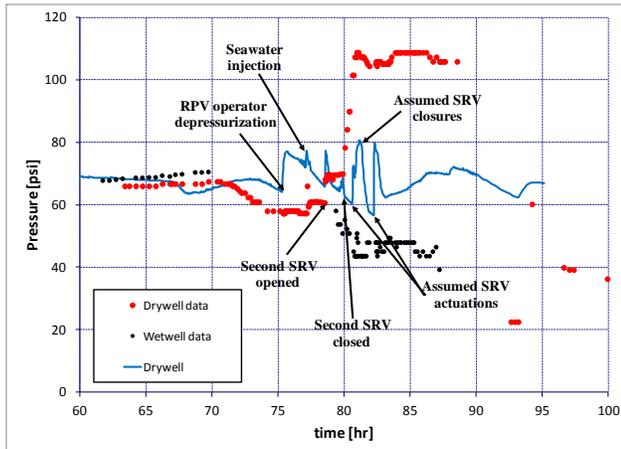
Fig. 10. Comparison between the containment pressure data and the analysis results for containment pressure given the assumed SRV operations.
