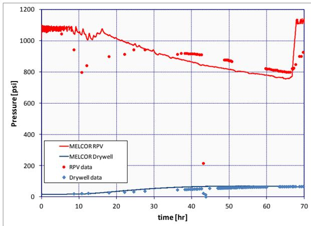
Fig. 4. Demonstrates the good agreement prior to RCIC failure of the system conditioning.
