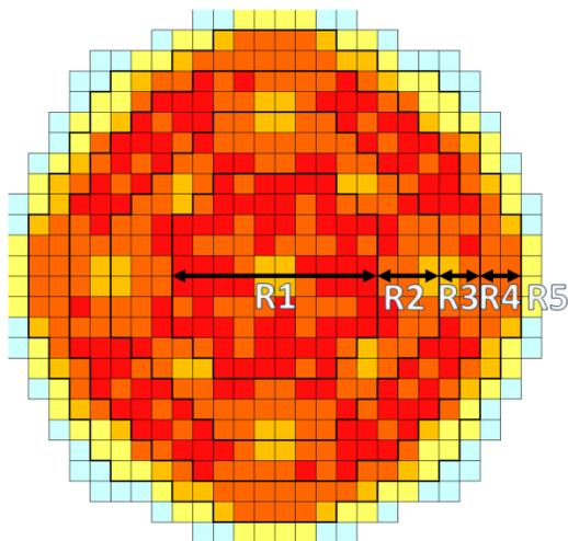
Fig. 3. Axially-integrated, assembly-wise power distribution for 1F2 with MELCOR core rings (post-processed TEPCO data, color contour legend omitted due to proprietary data considerations).
