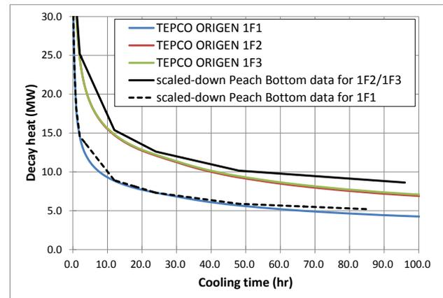
Fig. 2. Decay power vs. time after scram for 1F1, 1F2, and 1F3.
