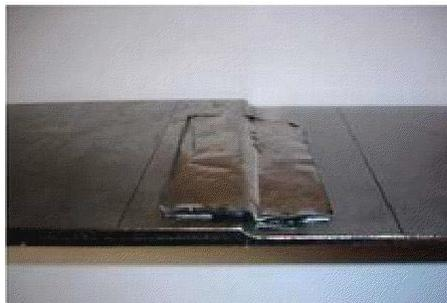
*Repair strip applied manually on lap weld.*
