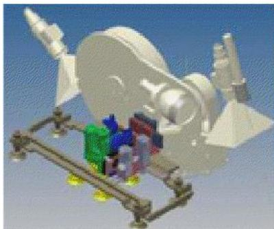
*General design of a robot able to apply repair strip*
