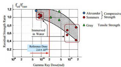
Figure 2 Compressive and Tensile strength of Concrete Exposed to Gamma Radiation  $f_{cu}$ , related to Compressive Strength of Untreated Concrete,  $f_{cu0}$ <sup>(1)</sup> (Legend symbols were changed and some notes were added to the original.)
