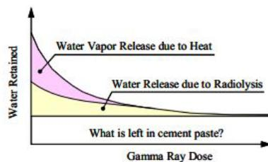
Figure 8. Gamma Ray Dose vs. Water Retained in Concrete.
